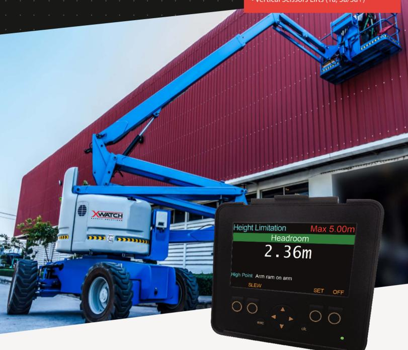
The XW MEWP can be configured to work on a variety of powered access equipment (MEWPs). Height and slew limitation is controlled using motion cuts providing accurate and repeatable performance without detriment to the machine.
