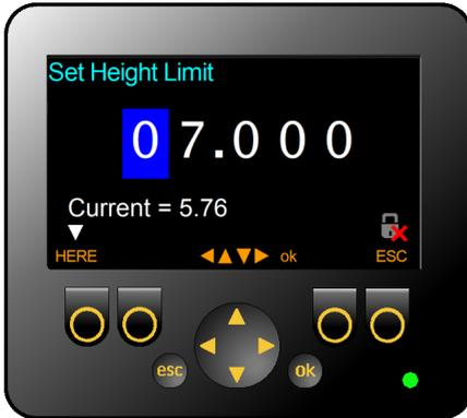
To automatically set a new height limit, move the machine until the desired height is achieved (shown as **Current = 5.76** in this example) and press **HERE**.
