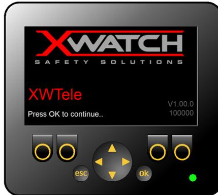
The system will start automatically when the machine ignition is switched on. After a short delay, while the system transfers information from the I/O controller, the display above will appear. The height limiter will operate after 10 seconds, or immediately if **ok** is pressed. Previous settings will be active.
