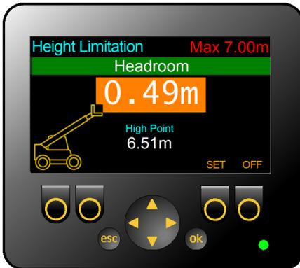
As the Headroom reduces to less than 0.5 metres, the headroom value displayed will change colour. Machines that are equipped with proportional motion control valves will reduce the boom up and telescope out speeds.
