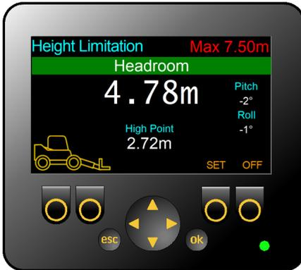
**Pitch** is the fore-aft chassis angle.
