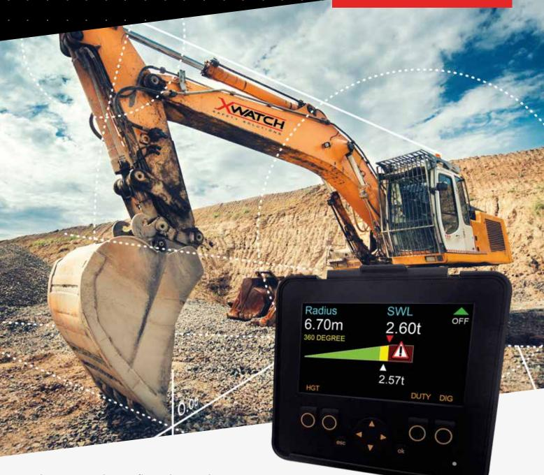
The XW2 can be configured to work on any type of hydraulic excavator. Overload and height limitation is controlled using proportional soft-stop hydraulic valves providing accurate and repeatable performance without detriment to the machine. A basic dig depth monitor is available when the RCI is not required. If hazards arise, XW2 will automatically flip to the relevant display page.
