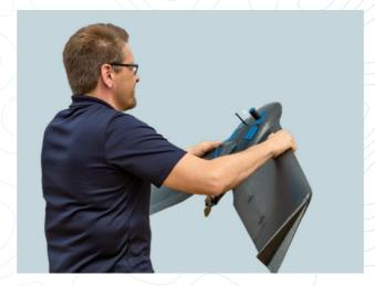
Upload your flight plan wirelessly to your drone. After a simple hand launch, your eBee Geo drone will then fly, capture images and land by itself.
