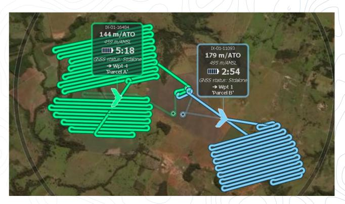
With eMotion, flights are built using mission blocks. Just choose your block, highlight the region you want to map, define key settings, and eMotion auto-generates your drone's flight plan. Multi-flight missions are supported and you can activate/import elevation data for even safer, terrain-accurate flights.
