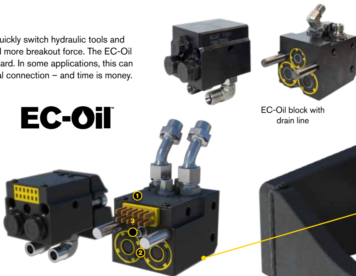
EC-Oil block with: 1. Electrical connector, 12 pole 2. Two oil connectors (supply and return) 3. Central lubrication
