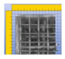
C-thrue visualisation: dual antenna polarisation allows the optimal detection of both first and deeper levels of rebars
