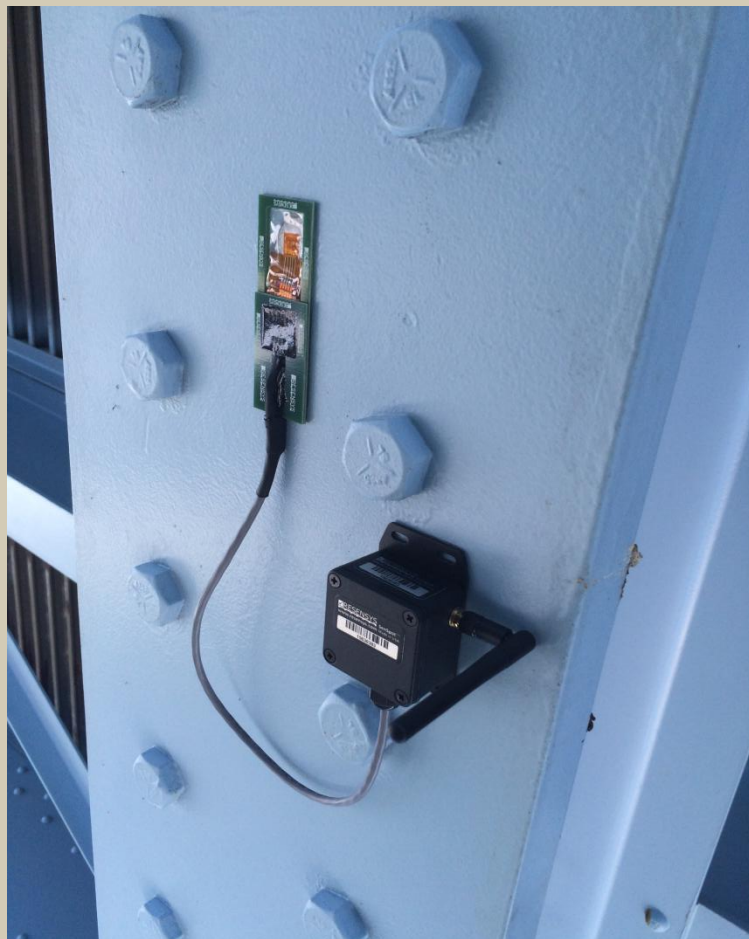
Resensys SenSpot™ sensors monitor 10,000-foot Robert Norris Bridge, Virginia
