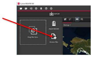
3.5. "Import BLK360" will launch a new Cyclone REGISTER 360 window that will allow you to connect to a local BLK360 Imaging Scanner and select individual files to import.
