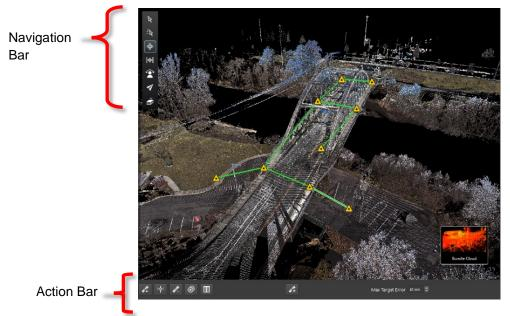
7.8. At any point, the user may access their "Settings" by clicking on the gear icon at the very top left of the screen to change units and set the error threshold for green, yellow and red links.
