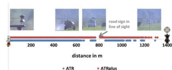
Figure 10 - Following and measuring on a prism under sunny conditions.
