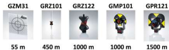
Figure 7 - Achievable ranges 1 for automated target aiming (static).
