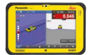
Leica iCON CC80 Rugged lightweight, powerful field controller.
