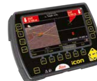
Leica iCON excavate iXE3 3D Excavating solution Full visual guidance of the bucket – see the job as you want. Menu keys give the operator an easy overview of functions.
