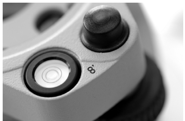
Figure 4 - Detail view of the GDF121 circular bubble
