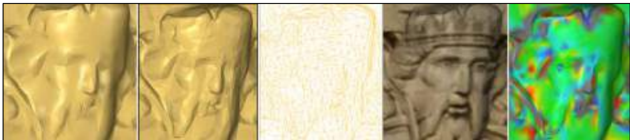
Figure 6: Representation mode on a mesh (from left to right: smooth, flat, wire, texture, inspection)
