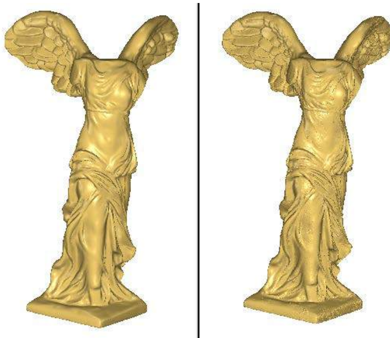
Figure 35: Comparison between the two refinement methods; Left: Interpolate new points; Right: Take points of the cloud
