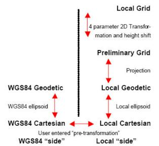
Note, when using a TwoStep transformation it is not possible to see the "preliminary grid" coordinates either in LGO or on the System1200 instruments. Only the final local grid coordinates are shown. This is correct since the "preliminary grid" coordinates have no practical use.
