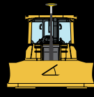
Single GPS & Slope Control
